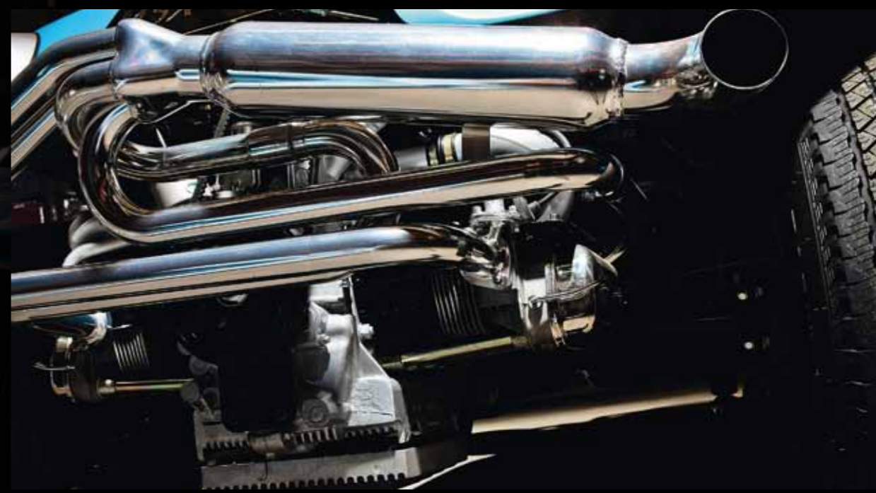
> 1600cc twin-port motor has been rebuilt by Alex Bruce to stock specs and 'sensibly' detailed. It uses a Split Bus oil bath air cleaner and deep sump as it will see plenty of heat and sand in Tenerife. Both cars have chromed Manx Sidewinder exhausts
