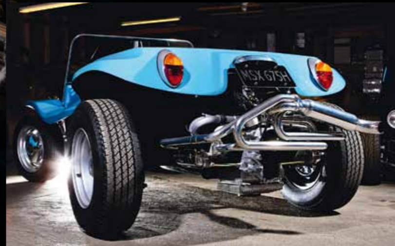
> 1600cc twin-port motor has been rebuilt by Alex Bruce to stock specs and 'sensibly' detailed. It uses a Split Bus oil bath air cleaner and deep sump as it will see plenty of heat and sand in Tenerife. Both cars have chromed Manx Sidewinder exhausts
