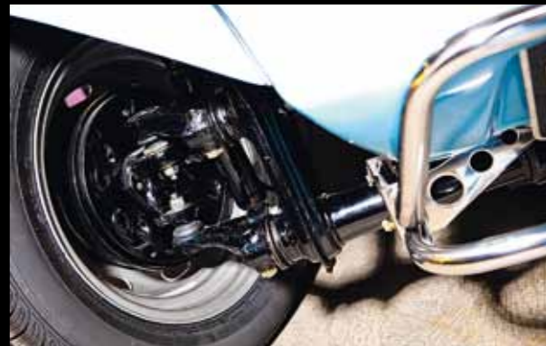
▲ Stock balljoint axle has been rebuilt with all new parts for longevity, and adjusters to fine tune the tyre-to-wheelarch gap. Polished stainless front nudge bar was a later addition requested by the car's owner
