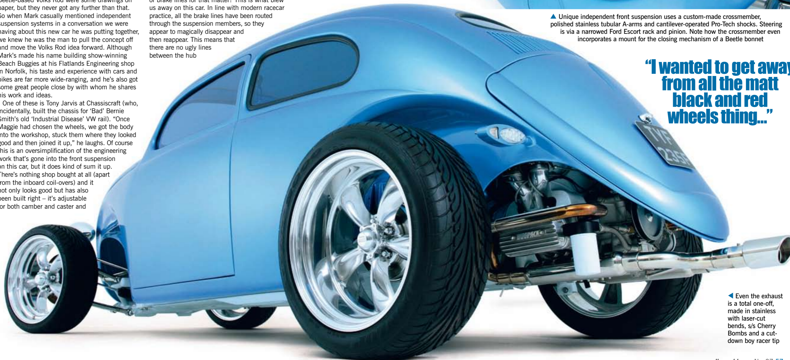
▲ Our favourite bit is the brake lines that run from the crossmember, through hard lines in the A-arms...
