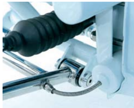
▲ Our favourite bit is the brake lines that run from the crossmember, through hard lines in the A-arms...
