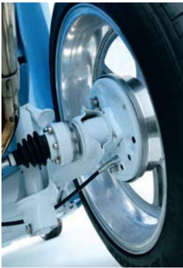
▲ IRS pan had its trailing arms swapped side for side, then the halfshafts chromed
