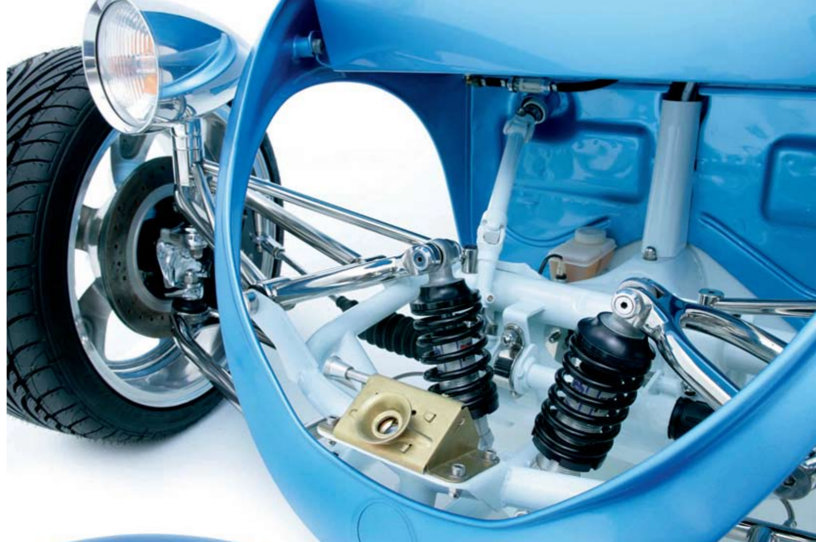
▲ Unique independent front suspension uses a custom-made crossmember, polished stainless tubular A-arms and cantilever-operated Pro-Tech shocks. Steering is via a narrowed Ford Escort rack and pinion. Note how the crossmember even incorporates a mount for the closing mechanism of a Beetle bonnet
