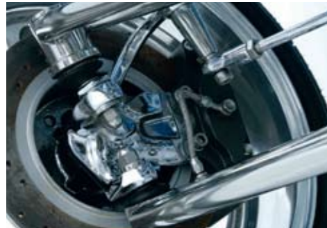
▲ ...and pop out the other end near the heavily reworked VW hubs. Front brakes are Tarox six pots
