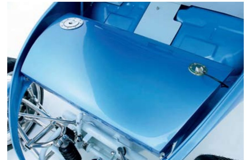
▶ Now that's what we call a custom-made fuel tank! What you can't see from here is the special cut-out in the back to house the fuel pump, or the fact that all the car's wiring is hidden behind the dash and then runs down through a conduit into the framehead
