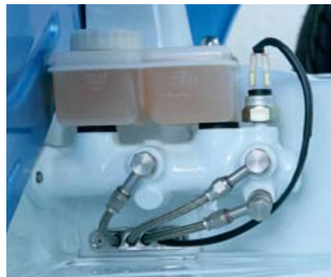
▲ Mark's favourite bit is this neat manifold into the framehead that takes all the brake lines and wiring
